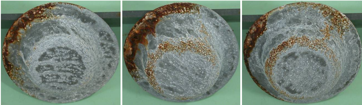
Figure 123 Formed HD ZnAlMg 10 μm after 18 weeks in ACT
