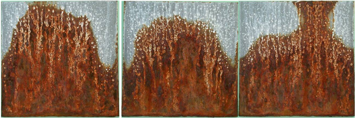
Figure 129 Flat GI 10 \mu\text{m} after 18 weeks in ACT
