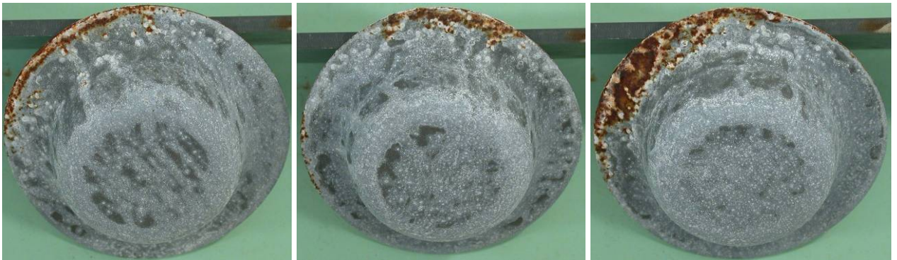
Figure 124 Formed HD ZnAlMg 14 μm after 18 weeks in ACT
