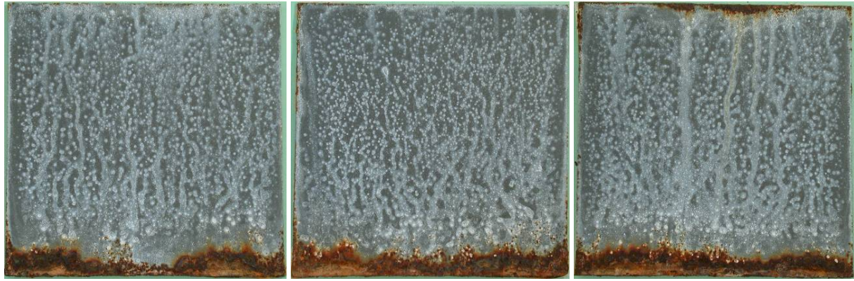
Figure 133 Flat HD ZnAlMg 10 \mu\text{m} after 18 weeks in ACT
