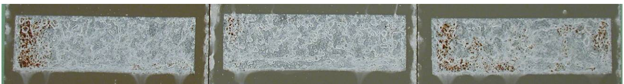
Figure 111 Galfan 20 \mu\text{m} in open configuration after ACT
