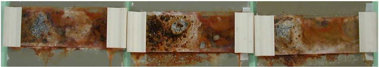
Figure 106 HD ZnAlMg 7 \mu\text{m} in Volvo crevice configuration after ACT
