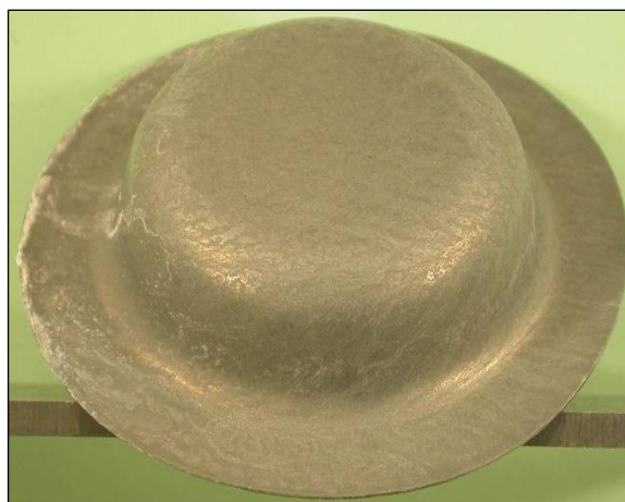
Figure 4: Photograph of a formed panel (after one week in the Volvo test cycle)
