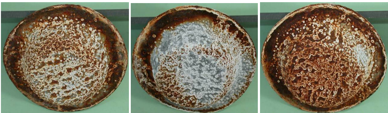
Figure 121 Formed Galfan 20 µm after 18 weeks in ACT
