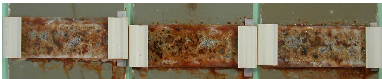
Figure 104 GI 10 µm in Volvo crevice configuration after ACT
