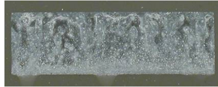
Figure 114 HD ZnAlMg 14 μm in open configuration after ACT
