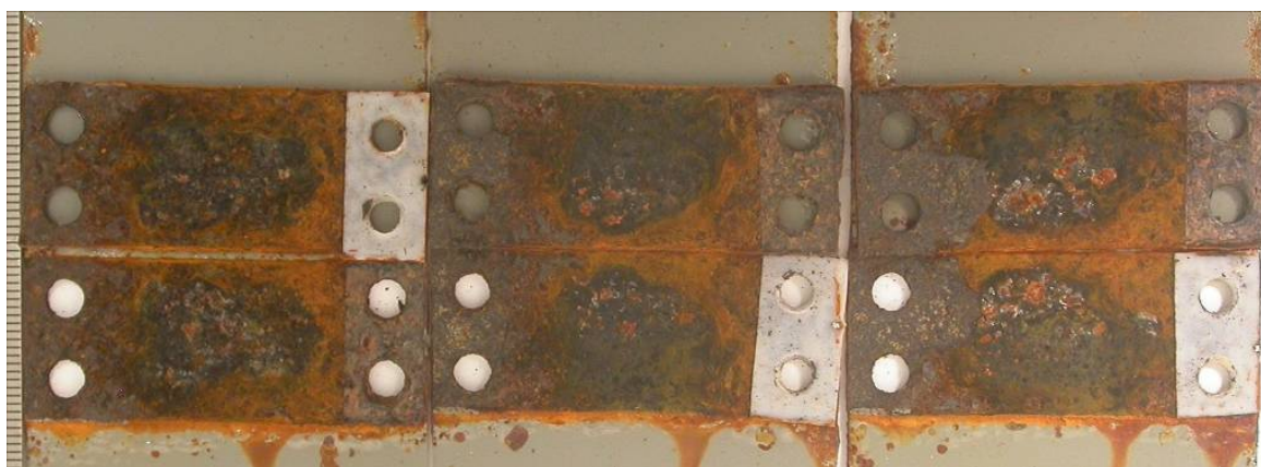
Figure 92 CRS Renault crevice panels after 6 weeks in ACT test
