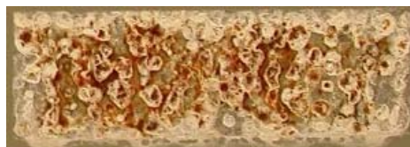
Figure 110 GI 20 \mu\text{m} in open configuration after ACT
