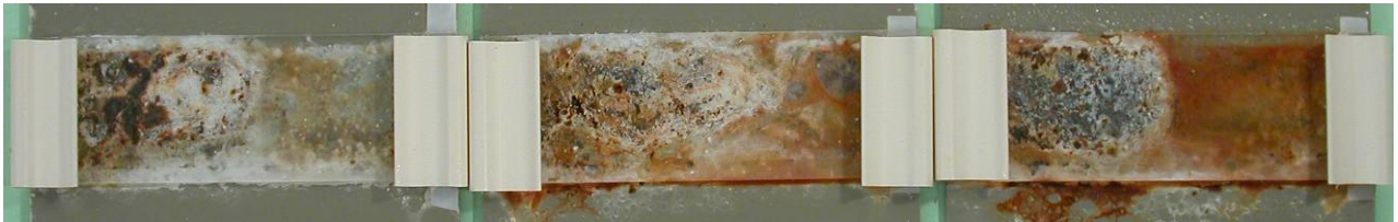
Figure 107 HD ZnAlMg 10 \mu\text{m} in Volvo crevice configuration after ACT
