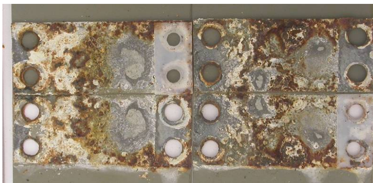
Figure 93 GI Renault crevice panels with the coating thickness of 10 \mu\text{m} after 6 weeks in ACT test
