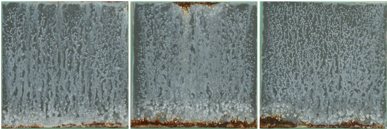
Figure 134 Flat HD ZnAlMg 14 \mu\text{m} after 18 weeks in ACT
