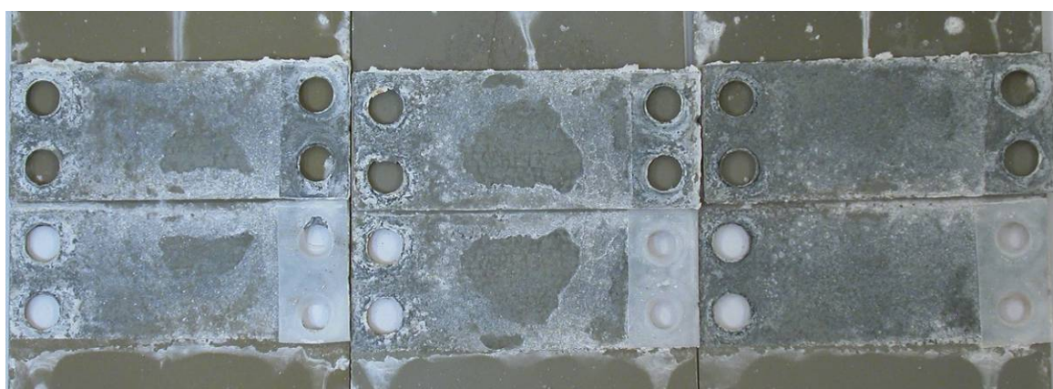
Figure 95 Galfan Renault crevice panels after 6 weeks in ACT test
