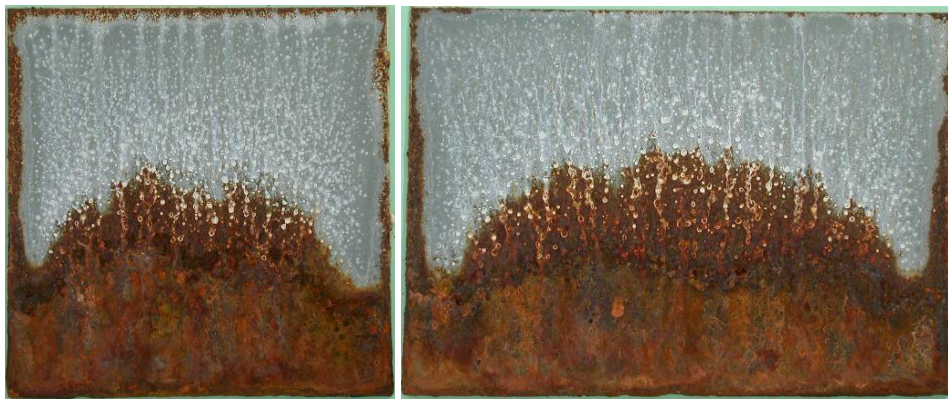
Figure 130 Flat GE 10 \mu\text{m} after 18 weeks in ACT
