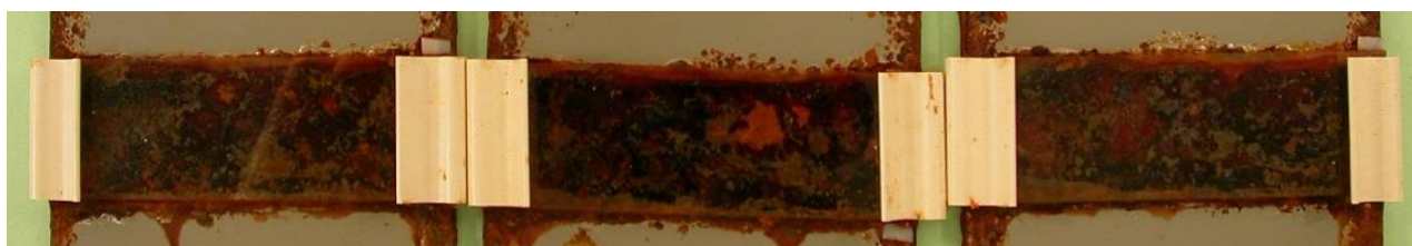
Figure 103 CRS in Volvo crevice configuration after ACT
