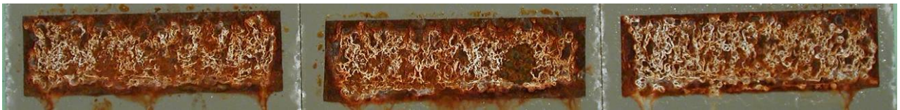
Figure 109 GI 10 \mu\text{m} in open configuration after ACT
