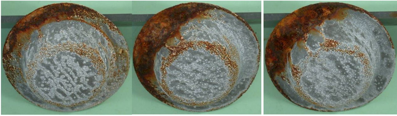
Figure 122 Formed HD ZnAlMg 7 μm after 18 weeks in ACT
