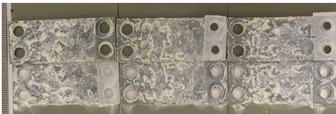
Figure 94 GI Renault crevice panels with the coating thickness of 20 \mu\text{m} after 6 weeks in ACT test
