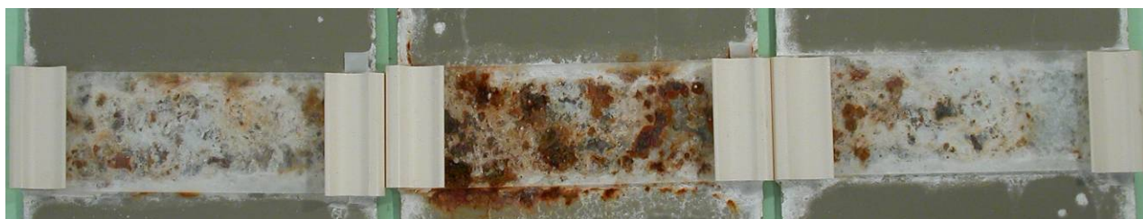
Figure 105 Galfan 20 µm in Volvo crevice configuration after ACT
