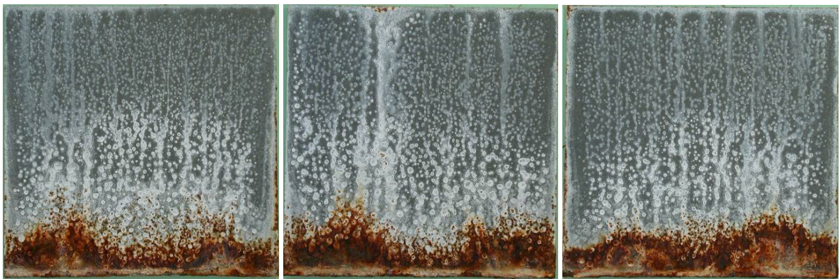
Figure 131 Flat Galfan 20 \mu\text{m} after 18 weeks in ACT
